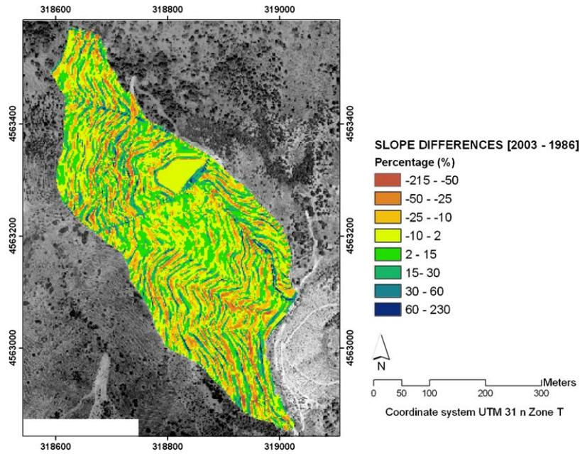
Fig. 5. Map of the slope degree differences between 1986 and 2003 in the sample field study area.
